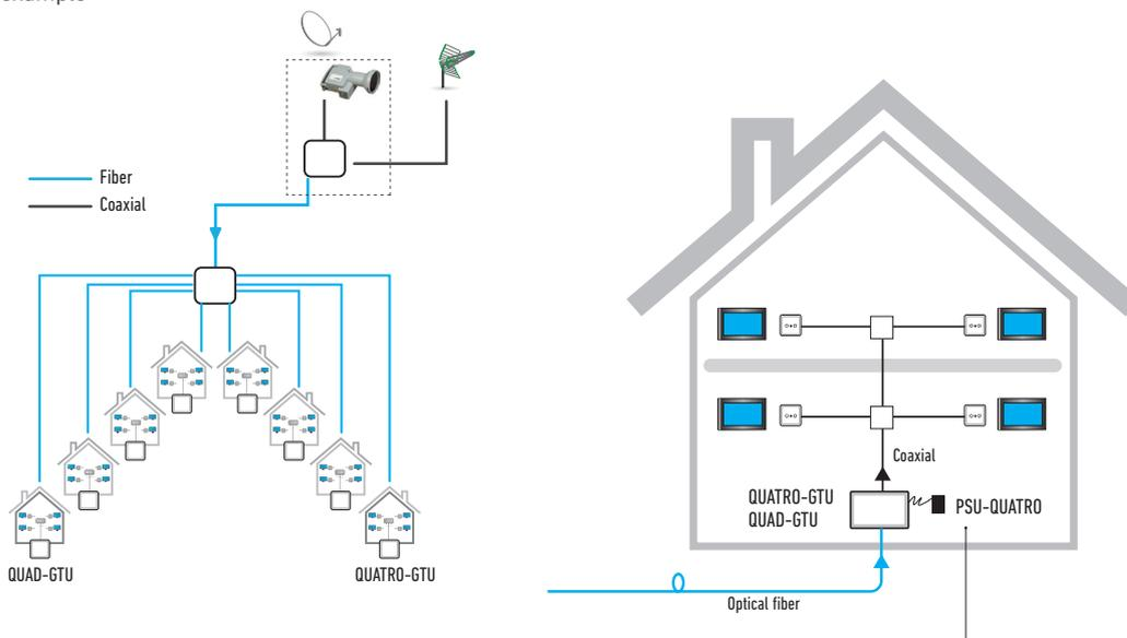
If there is no power supply or if the current supplied is not sufficient to power the QUATRO or QUAD optical receivers, the external PSU-QUATRO power supply unit (4951) must be fitted.
